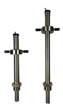
The GF 2552 Metal Magmeter from Georg Fischer features all-stainless steel construction. The PVDF nosepiece and FKM 0-rings are the only other wetted materials. The 2552 installs quickly into standard  $1\frac{1}{4}$  in. or  $1\frac{1}{2}$  in. pipe outlets, and is adjustable to fit pipes from DN50 to DN2550 (2 to 102 in.). Two sensor lengths allow maximum flexibility to accommodate a variety of hardware configurations, including ball valves for hot-tap installations.
